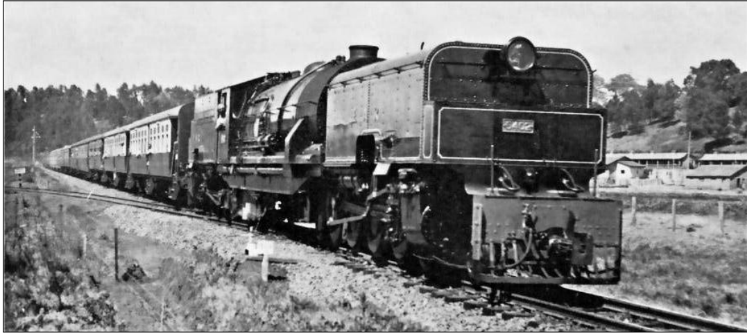
Above: Archie Morrow's third Garratt, #5402. The caption to the original photo reads "KUR class EC4 4-8-2+2-8-4 EAR No 5402 the last in service, with the down mail at Limuru Station" Photo from "Steam Locomotives of the East African Railways" by R .Ramaer
