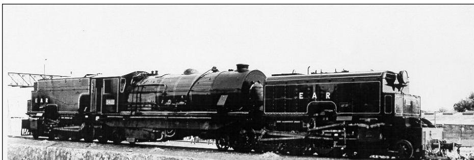
Archie Morrow's first Garratt, East African Railways #5302. (Chris Greville collection). This engine was a GA (later 53) Class Garratt delivered to Tanganyika Railways in 1939.
