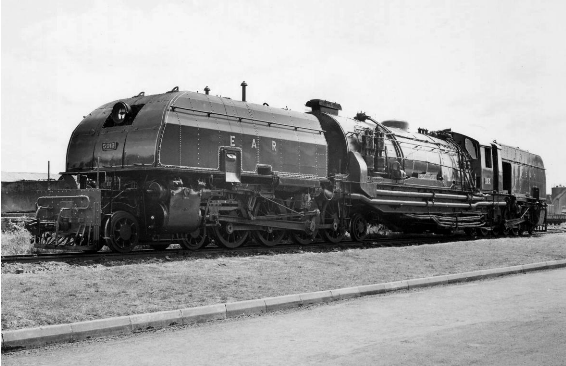
[ABOVE: 59 CLASS NO. 5913 – MOUNT DEBASIEN, OUTSHOPPED AT NAIROBI WITH A GIESL INJECTOR]
