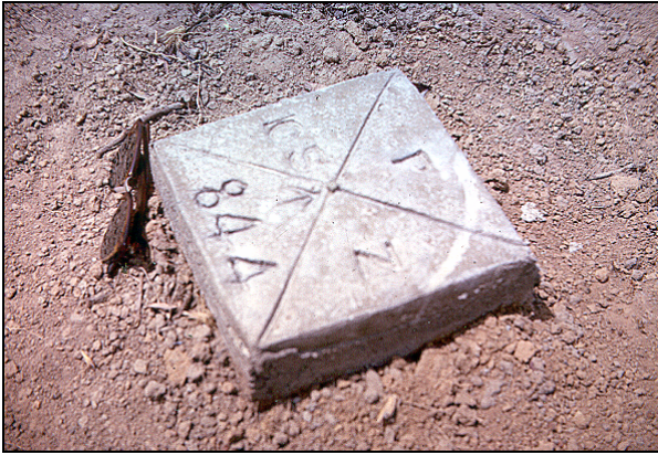
70. Primary cadastral control beacons were generally pre-cast concrete pillars about 2' 6" long and 9" square in section, with a 4" nail sunk to its head as the centre marker, and bearing a unique reference number.
