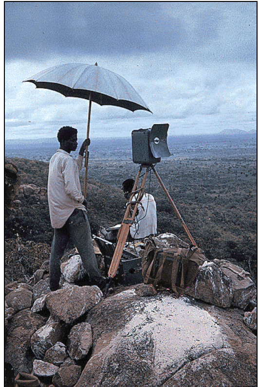
50. At Dutsen Wai in Zaria Province in 1963, establishing framework control for the West Kano block of topographic
