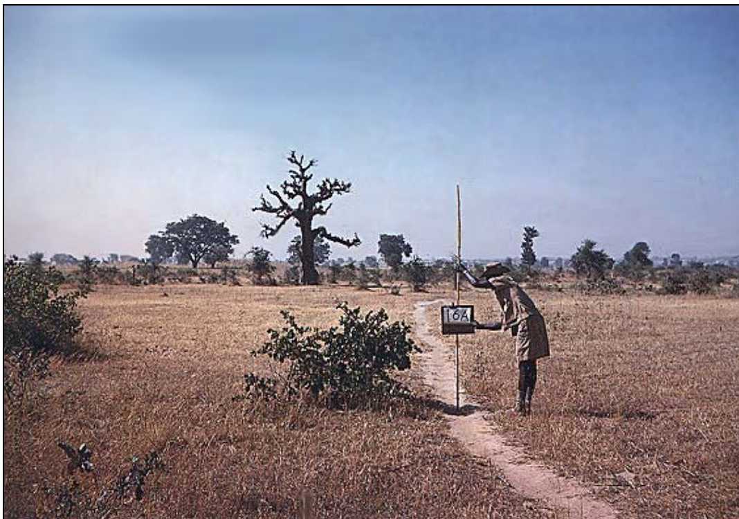
64, 65. Two of the photopoints selected to control stereo models for the 1:2,400 scale mapping of Gusau in Sokoto Province in 1962.
