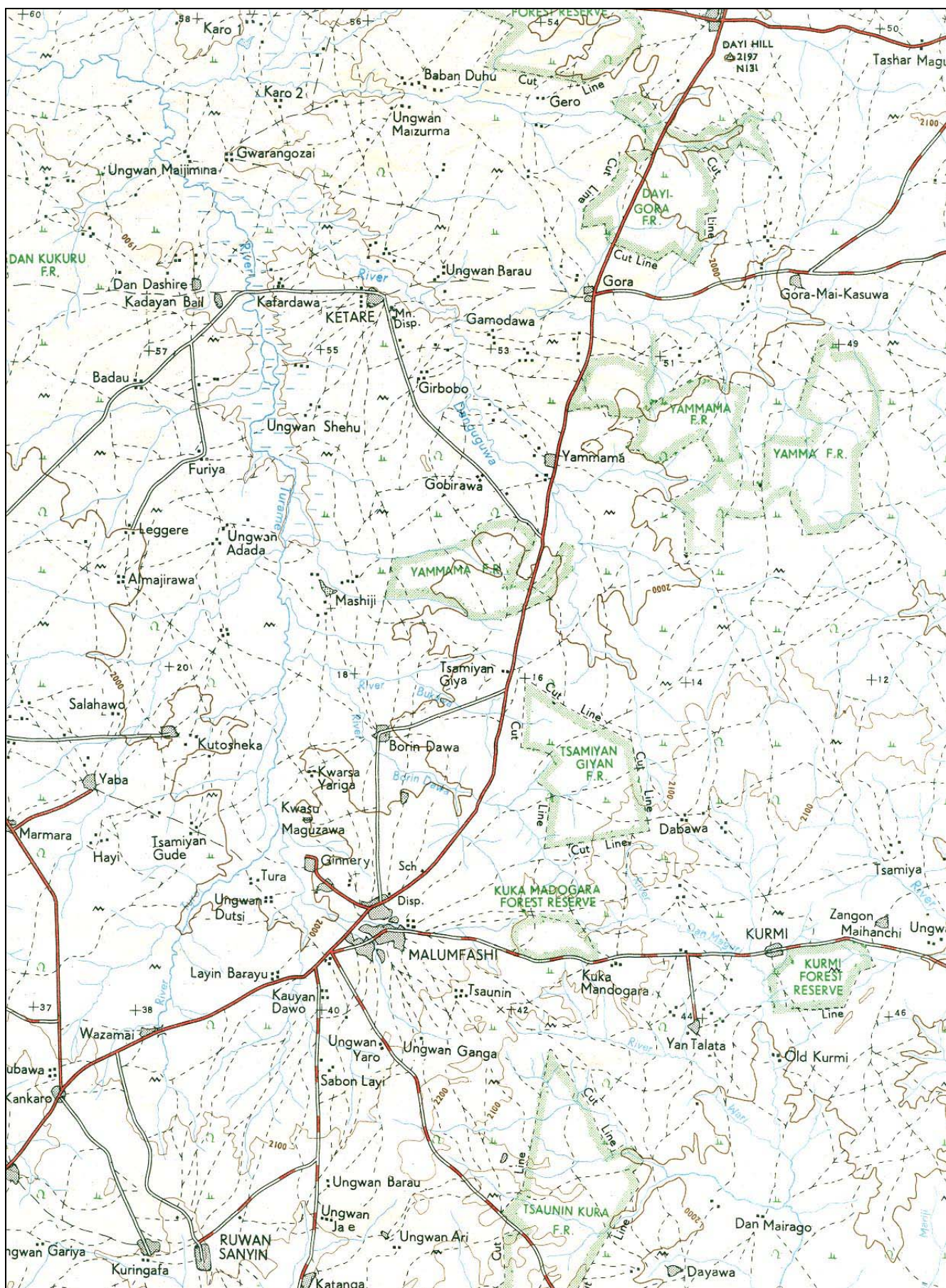
M27. A reduced scale extract from the first edition 1:100,000 scale Malumfashi Sheet 79, showing parts of the North-Central and Kano States with contours at 100 ft vertical intervals. This map was compiled, drawn and first printed by the Interim Common Services Survey Unit at Kaduna in 1969-70 from photographic reductions of 1:50,000 scale maps. Control and ground information was supplied by the Northern Nigerian Survey and the air photography obtained by Hunting Surveys Limited in December 1963.
