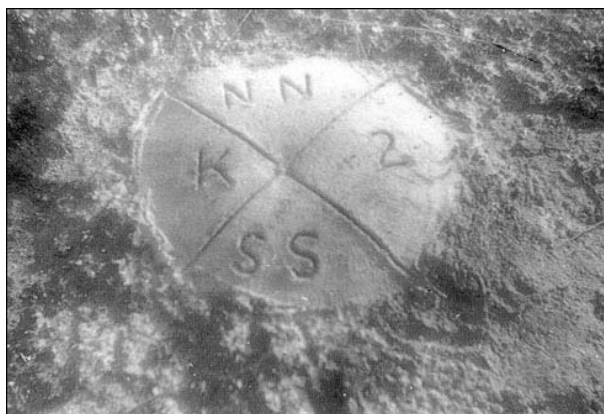
31. The ground marker for the K2 trig point, set in rock
