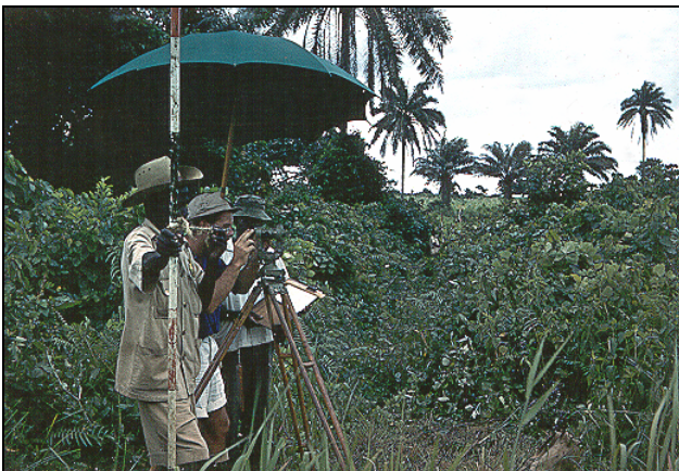
72. Malcolm Anderson, catenary taping along a cleared line for the control survey of Offa, Ilorin
